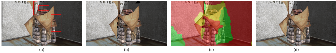
Figure 1: (a) Scene rendered by adaptively blending four forward-warped images as proposed by Stich et al. The image shows ghosting artifacts (red boxes) and appears blurry. (b) Our proposed graph-cut interpolation algorithm. Black areas indicate holes that are invisible in all input cameras. (c) The image overlaid with the optimal labeling, each color denotes a different source image. (d) Final result, invisible regions are filled by spatio-temporal image inpainting.
